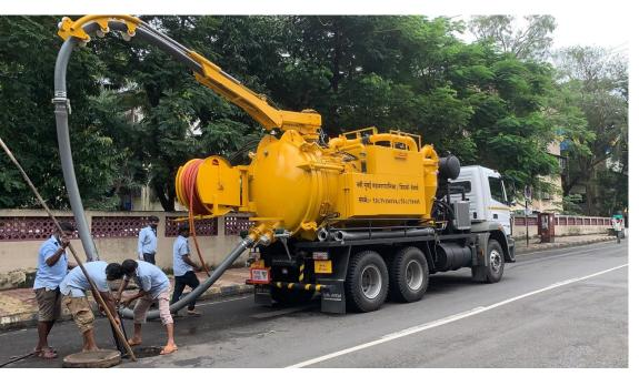
Our KAMBI Hi Flow of 12,000 Lt capacity makes its way through Navi Mumbai performing the vital job of preventive maintenance of sewer lines.
